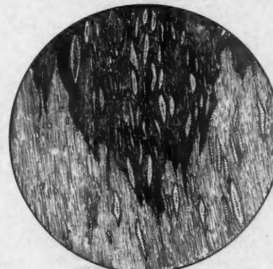
FIGURE 14. INTENSELY DEFORMED SHALY LIMESTONE WITH SCATTERED OIDS AND CONTORTED BEDDING PLANE Deformation beyond measurement. Spec. 325, 3 1/4 miles southwest of Mechanicsburg, Pa.
